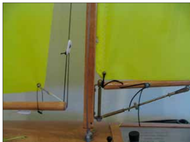
A Topping Lift attached to the end of the Jib Boom.
